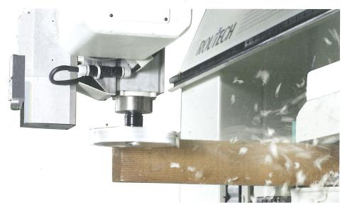
OIKOS RT4000, because of the independent 5-axis routing unit, goes beyond the conventional limits in the field of beam processing. OIKOS RT4000 allows the use of the same tool horizontally and vertically. Execution of rounded edges or profiling operations can also be performed with a single tool, in any angle and position. Boring operations and connection geometries in any shape, size and inclination are executed like a standard machining operation in the simplest way.
