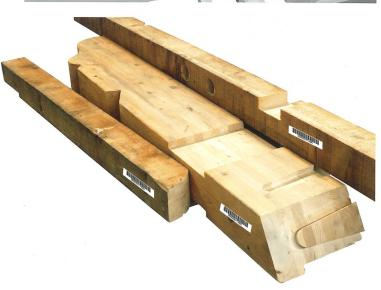
In view of the most efficient production process, it is also necessary to optimise the beam storage after outfeed of machine. The outfeed table of the OIKOS RT4000 is therefore fitted with an outfeed device to push the processed beam onto the storage station for off-loading by means of handling equipment. The machine can be equipped with markers and/or labelling devices to sign each single beam in order to facilitate the identification in the production department or on the building site.
