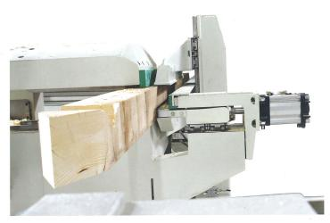
A second clamp provides the transport for the beam towards the machine outfeed.
