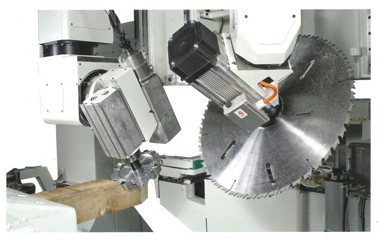
A simple idea was at the origin of OIKOS RT4000: Introduction of the flexibility of the machining centres into the production process of structural timber constructions. For this purpose, OIKOS RT4000 is equipped with flexible, versatile and efficient machining units:
