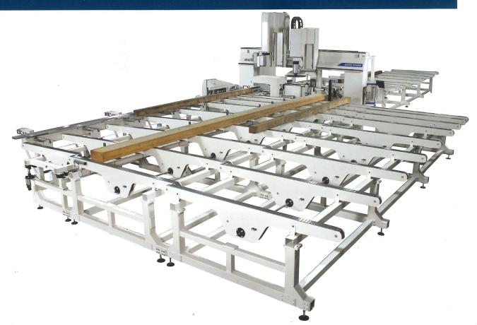
OIKOS RT4000 can be integrated with an automatic infeed system, thus allowing to load the machine without the constant presence of the operator.
