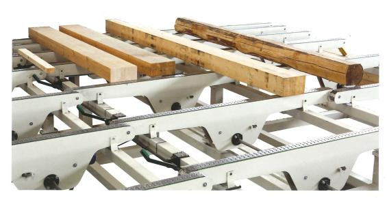
OIKOS RT4000 meets all production requirements, since it allows to clamp dimensions up to 800 x 300 mm and even special beams with rounded edges with a cross section of 350 x 350 mm.
