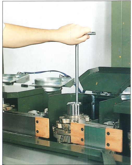
20 - Spindles are not counter-supported thus allowing an easy and simple access for tool change.
