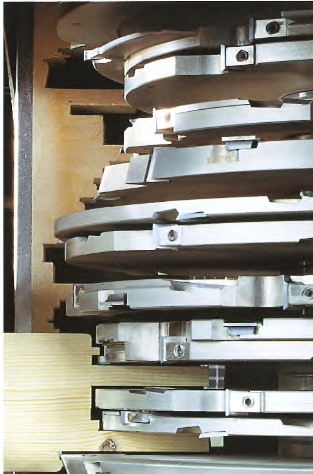
Spindle moulder H = 620 mm with Jolly/L automatic anti-chipping unit.
