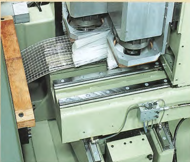
All Copytronic units are driven by brushless motors and have prism guides with automatic forced lubrication as standard.
