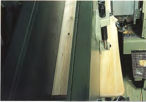
Corner rounding units. Fitted with electro-chucks (7.5 kW at 18000 rpm) with speed adjustment by static inverter. Available in routing and sanding versions.
