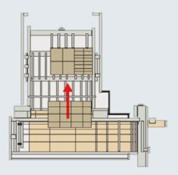
The crosscut section can be manually loaded and used as a normal single blade beam saw.
