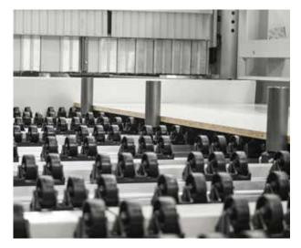
**POWERED SIDE ALIGNER** on prismatic guideways with recirculating ball bearings.
