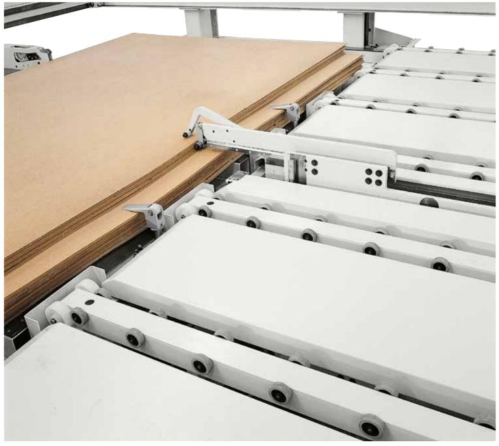
**AUTOMATIC LOADING SYSTEM OF THIN PANELS: SCM EXPERIENCE AT CUSTOMER DISPOSAL** Precise and effective device which ensures the automatic loading of thin panels with thickness ranging between 3 and 10 mm.
