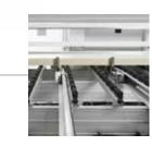
**Powered side aligner for cross cuts** Perfect alignment of the piece with a drastic cycle time reduction.
