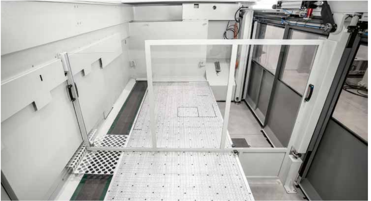
Possibility of dividing the worktable into two semi-tables with a central bulkhead, for pendulum machinings.
