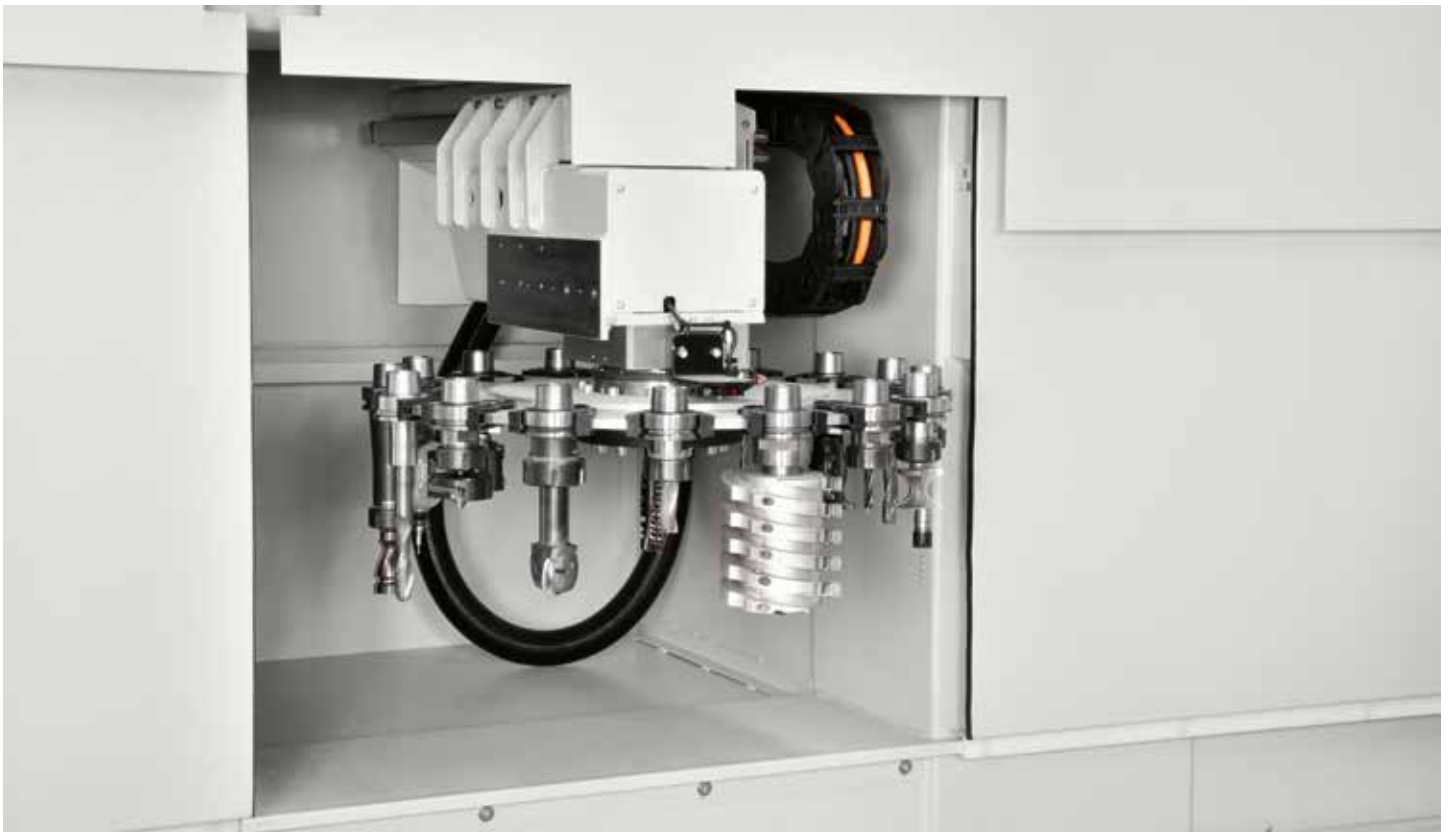
Circular tool store fitted with integral protection and rear access door for the manual tool change from the machine outside.
