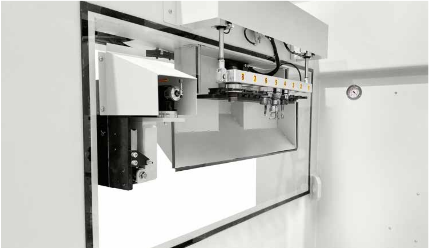
Minimized idle times with the “Pick-up” tool store installed on the machine left side.
