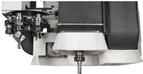
Higher efficiency and working time reduction with the additional routing unit (PBTC) with 12 kW electrospindle and Rapid 6-position tool changer to carry out the tool change in masked time.
