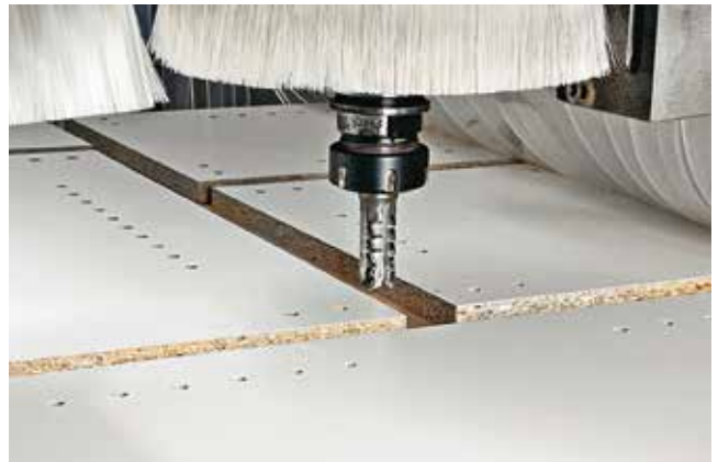
Possibility to work small work pieces with the coaxial mechanical presser.
