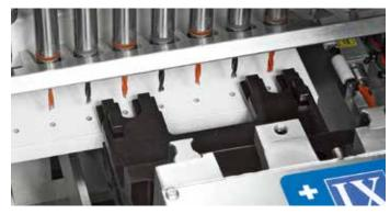
The panel hold-down grippers with X independent movement allow drilling and routing operations also in positions inside the gripper area thanks to new geometry, optimizing the re-clamping of the workpiece, reducing the cycle times and allowing to process on all 6 faces of the panel.
