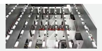
The work table is designed to perform all machining operations in the spaces between the supports. It is made of special rollers in a scratch resistant material, it guarantees the careful movements of the panels to ensure that the panel surfaces are not scratched. Rigid pressers at the infeed and outfeed to the work area, guarantee the positioning of the workpiece during the machining phase.
