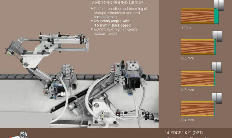
Automatic positioning of the group for the machining of 3 thin edges and 1 radius edge
