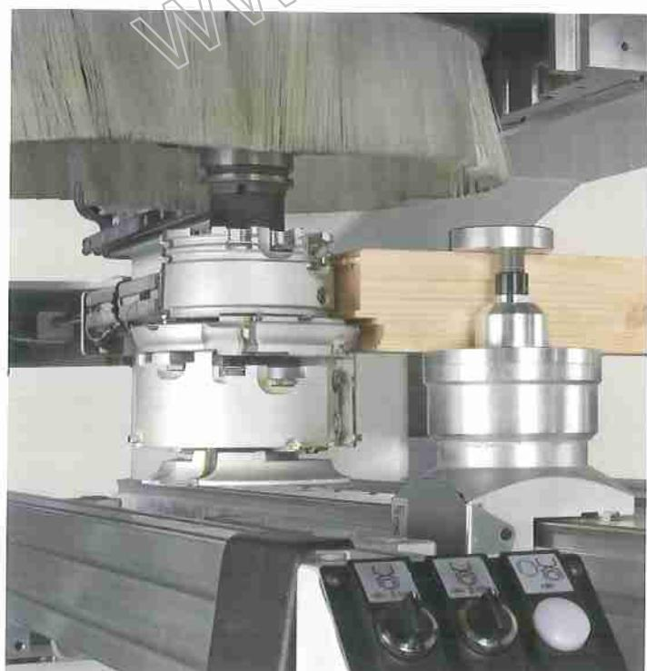
The TVN worktable with the height of 110 mm offers the great advantage of using double profile tools, reducing the number of tool changes and greatly increasing productivity.
