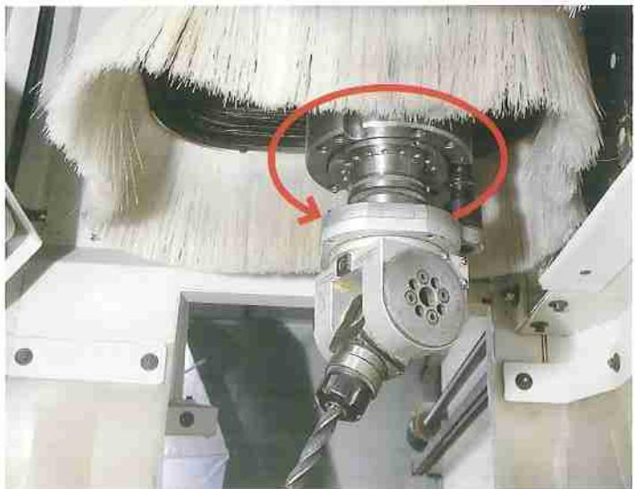
Record 100 NT is arranged for the use of angular driven heads so, as it has the interpolating Vector rotating axis (0-360°) for less tool changes thus providing increased productivity and accuracy.
