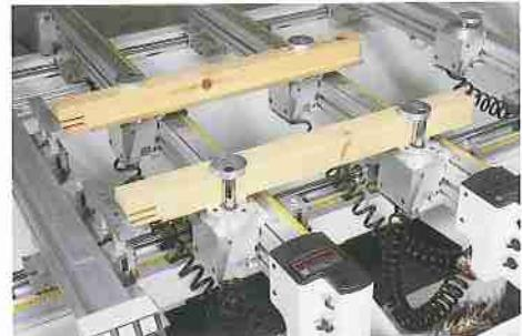
TVN SET is the ideal worktable for the automatic positioning of the bars for linear components such as doors, windows, staircases, beams, and columns. Extremely simple and easy to use, this system combines the flexibility of clamping device manual positioning with automatic bar positioning handled by the CNC.
