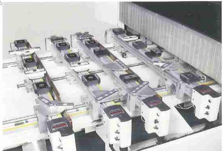
If suction-cups are not enough for component clamping, pneumatic clamps with a quick release system on the bar side are available.
