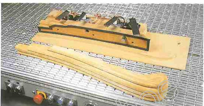
Inverted "T"-shaped grooves and a series of threaded holes provide perfect fixing for all hold-down devices.
