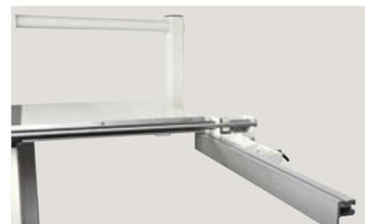
The rip fence has a cast iron body, extruded aluminium rule, and slides on a wide steel bar: there is no compromising on quality. The whole worktable can be easily and completely retracted.
