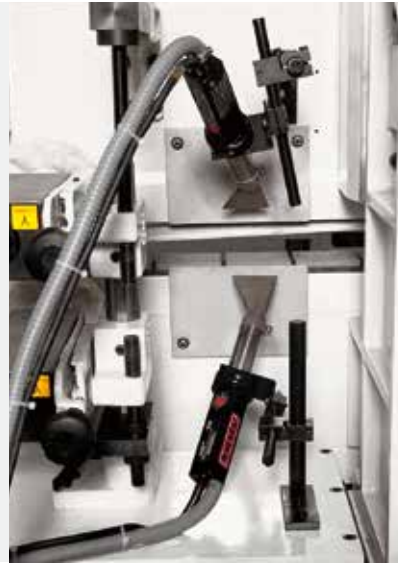
EDGE BRIGHTENING UNIT PH/1600 To finish plastic edges. xd
