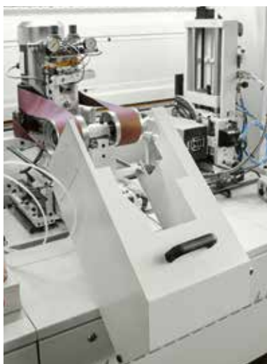
SANDING UNIT GLC For finishing and preparation of veneered and solid wood edges for painting. md xd
