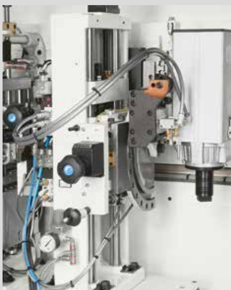
TOUPIE U Unit with vertical and front feelers – 90 mm 2 max groove section md xd
