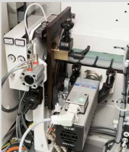
TOUPIE K-100 Unit with front feelers – 60 mm 2 max groove section kd
