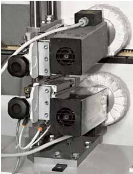
BRUSHING UNIT SPF To clean the panels and brighten plastic edges. xd
