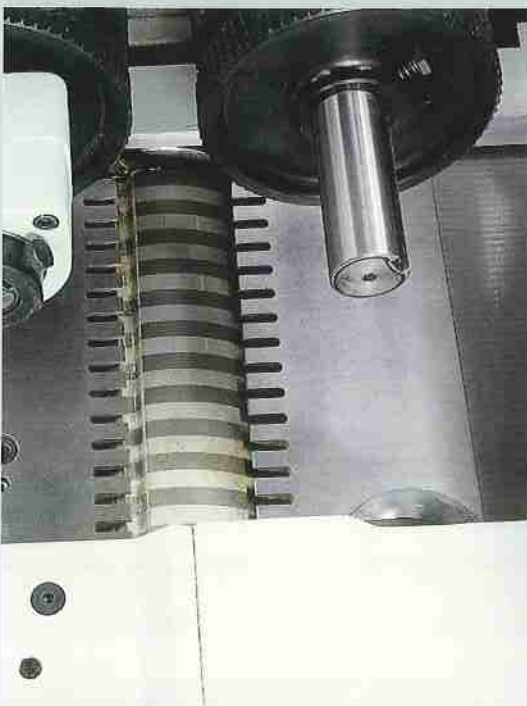
Quick release top feed roller and horizontal pressure roller before planer spindle
