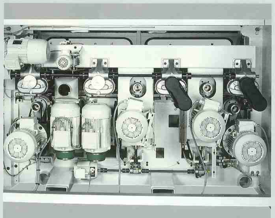
Independent motor for each spindle. Standard spindle power 5,5 kW (7,5 HP)
