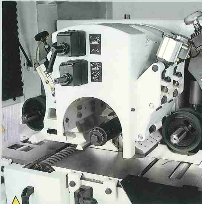
Powered feed rollers in worktable
