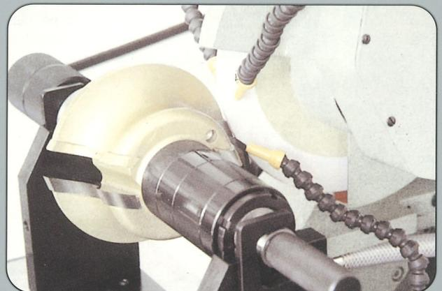
Sharpening and profiling of blades, cutters, bits and HM inserts.
