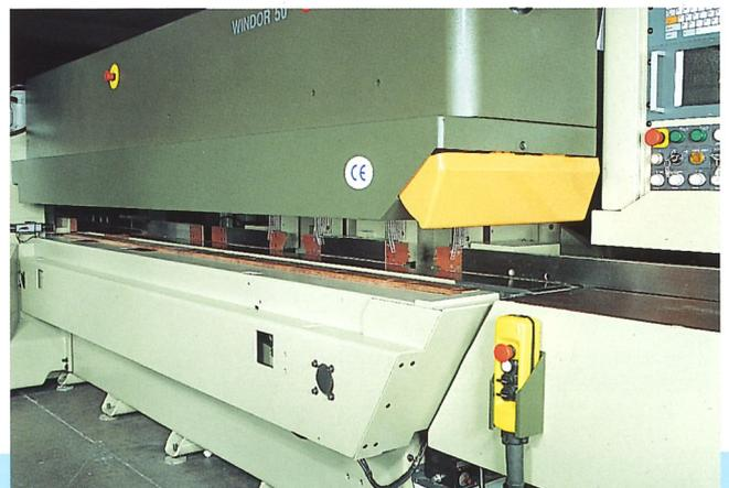
The WINDOR 50 moulder has multi-tool spindles able to machine a component on four sides in a single operation - maximum quality and precision, minimum down time.
