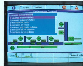
The programming of machining operations is very simple : all programming is CNC-guided and all the operator has to do is to answer the queries appearing on the display screen.
