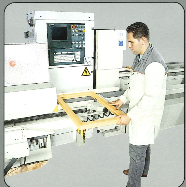
Lowering the glazing bead Abaissement de la pareclose
