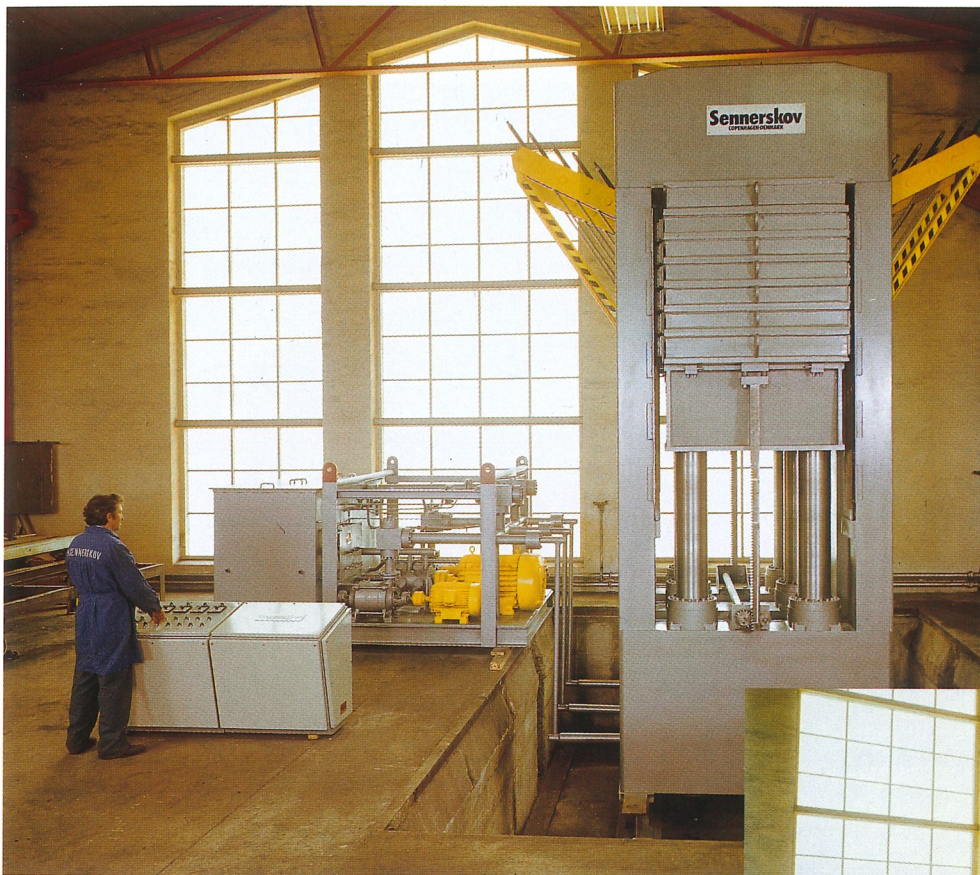
◀ 6-opening particleboard press with simultaneous closing system. Closed.
