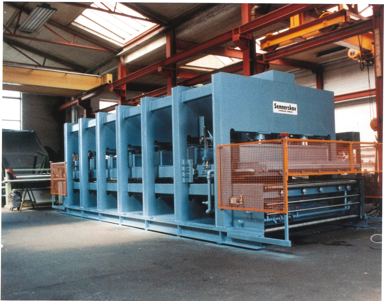
Single-opening downstroke hotpress for large size PUR-panels (shown press = 3 x 10 mtr.)
