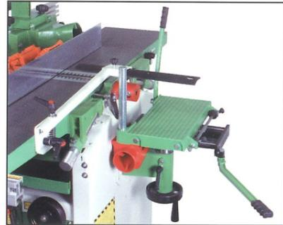
**IL GRUPPO SEGA – THE SAWING UNIT – DER SÄGEAGGREGAT
