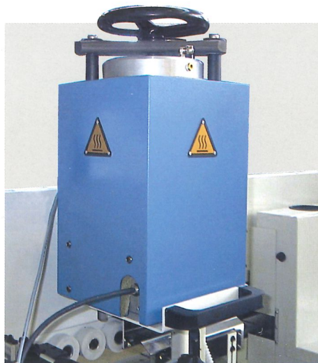
PUR glue process device Kit application colle polyuréthanique (PUR) Anbringungsakit Polyurethanleim (.PUR)
