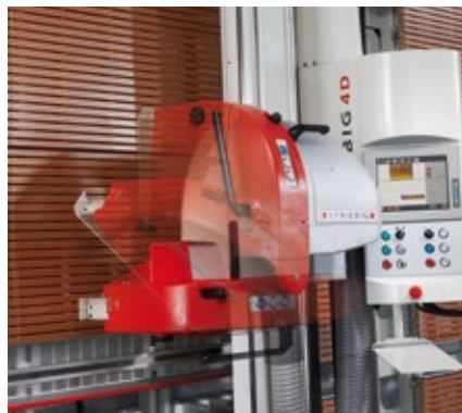
One of the numerous functions of the Striebig 4D: automatic motor swivelling. It assists the fully-automatic sawing procedure and makes work significantly easier for the operator
