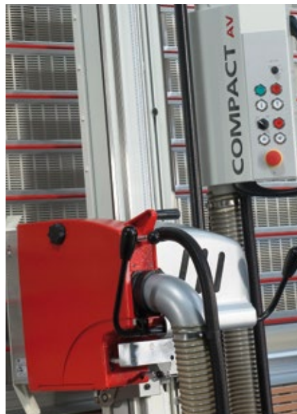
"Classic and prize-winning" Striebig design: saw unit and control box of the COMPACT AV. Ease of use has always been a Striebig trademark.
