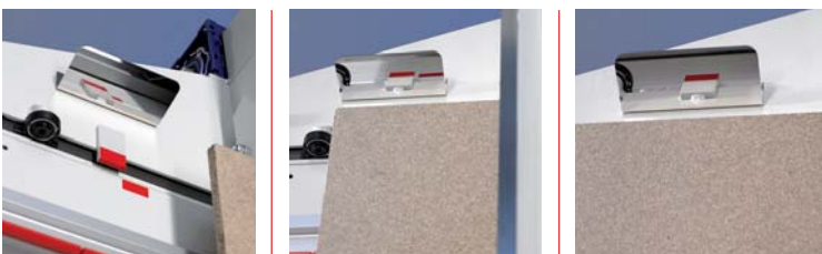
The mirror on the saw beam facilitates orientation with respect to the vertical cutting point (important to larger and overlaying panel sizes).
