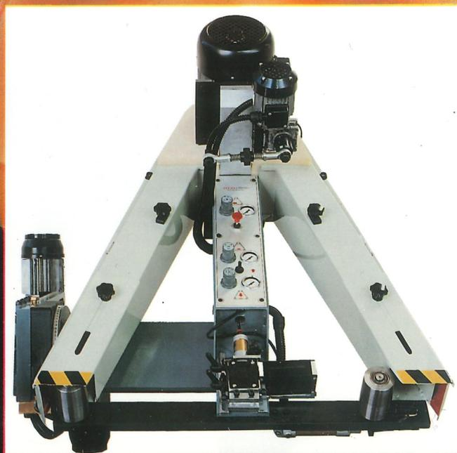
LEVIGATRICI PER BORDI E PROFILI MONOSPALLA  ONE-SIDED EDGE AND PROFILE SANDING MACHINES  PONCEUSES AVEC UN MONTANT POUR TRAVAILLER LES CHANTS ET LES PROFILS
