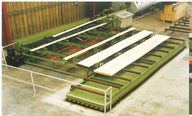
6. Layer stacker for efficient and reliable stacking of work pieces. The size of the pack is set by the operator. The finished pack can then be covered and strapped as required.
