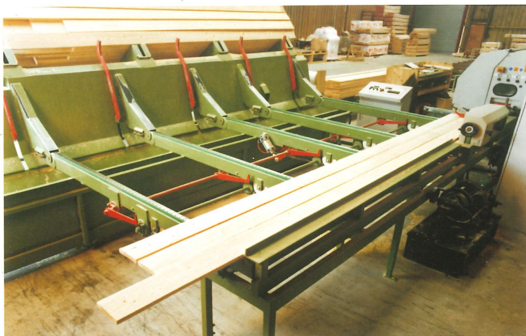
3. Automatic infeed to the moulding machine. Chain conveyors with a single piece feeding and powerful hydraulics ensure an efficient infeed to the moulder. As optional extra, the line can be equipped with manual rejecting.
