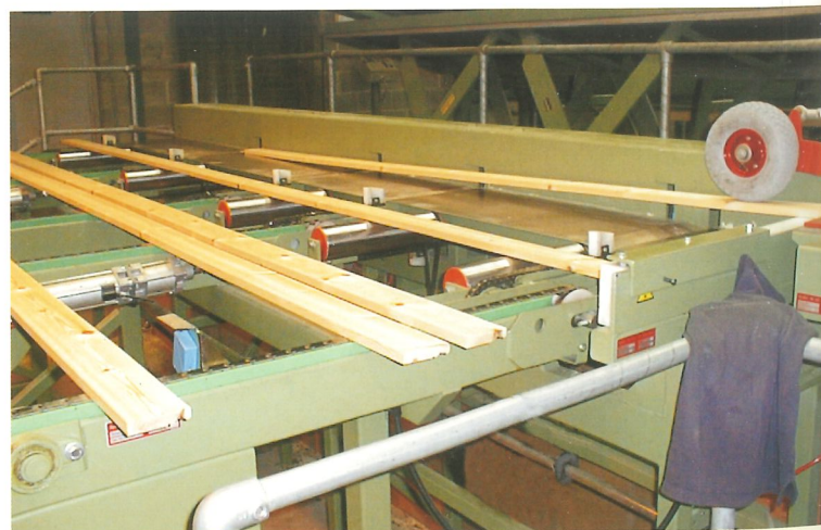
4. Outfeed from moulding machines. The stud carriers and fair ending rollers align the timber for a perfect finished pack. Tallying and inkjet marking can be incorporated.
