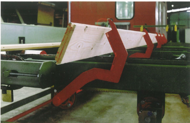
5. Programmable turning device for automatic turning of workpieces for visual inspection or for stacking of machined timber in a particular way.
