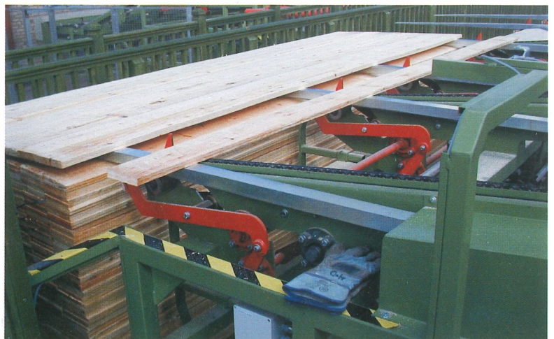
Layer stacker for efficient and reliable stacking of work pieces. After processing the work pieces are automatically and reliably stacked into layers forming a complete package.
