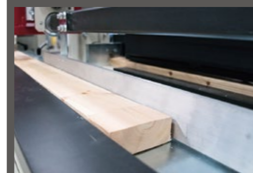
▶ Two channel press system to achieve high capacity. During final pressing of a workpiece, the subsequent workpiece is being prepared to ensure full utilization of the hydraulic press.
