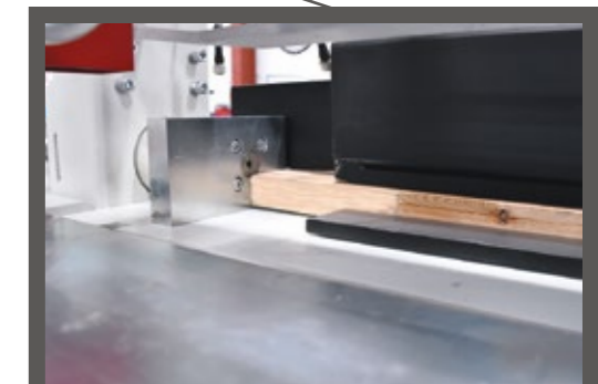
▶ Hydraulic press station for strong and correct press force. To keep workpieces from shifting position during the press process, they are supported by mechanical guiderails from all sides.
