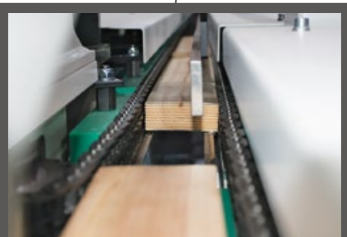
▶ Pre-alignment and buffer zone. Two high-speed guiding chains: one fixed and one moveable. Furthermore, top and bottom guiderails of stainless steel to ensure correct positioning of workpieces before pre-press.
