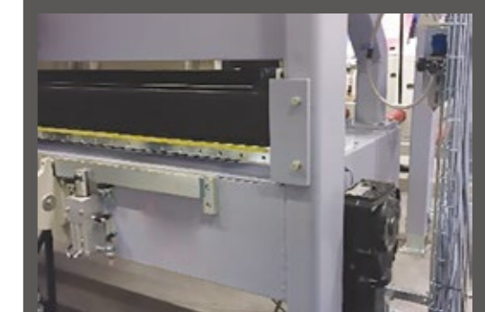
▶ Pre-press and press frame manufactured in heavy-duty design to prevent deflection during operations.
