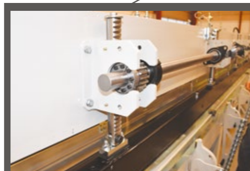
▶ Servo driven heavy-duty top bar, for minimum movement, correct pressure force, high capacity and easy to adjust/change from the operator panel.
