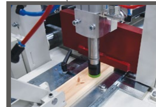
▶ Cross-cut saw which includes fixed positioning of the workpieces for the purpose of pre-cutting to lengths before press station.
