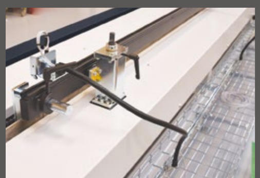
▶ Automatic variable speed regulation of pre-press based on the buffer size of workpieces. This ensures continuous high capacity flow, thus minimizing the occurrence of stops
