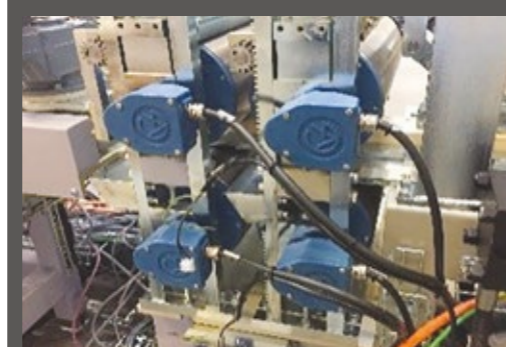
▶ Double set of top and bottom drum motors which include pneumatic brake units. These secure fast and reliable pre-pressing of all joints.
