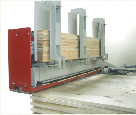
Stick magazines for dispensing of sticks to stabilise the packs.
