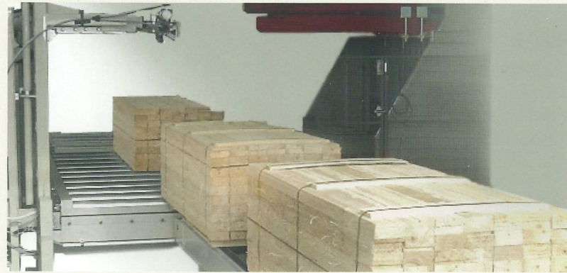
Example of automatic pack transport with bundling of packs. This leads to minimal time consumption by pack change, thus increasing the capacity of the plant.
