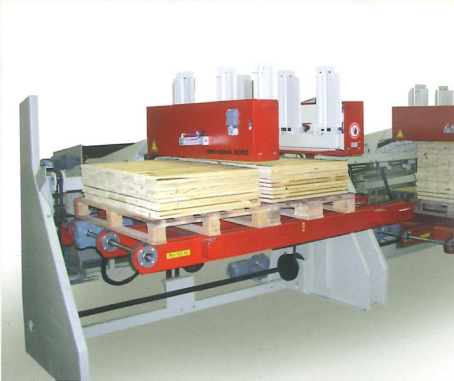
By stacking of short workpieces you may wish to completely fill a pallet. This can be achieved as shown in this example where more than two packs are stacked on one pallet.
