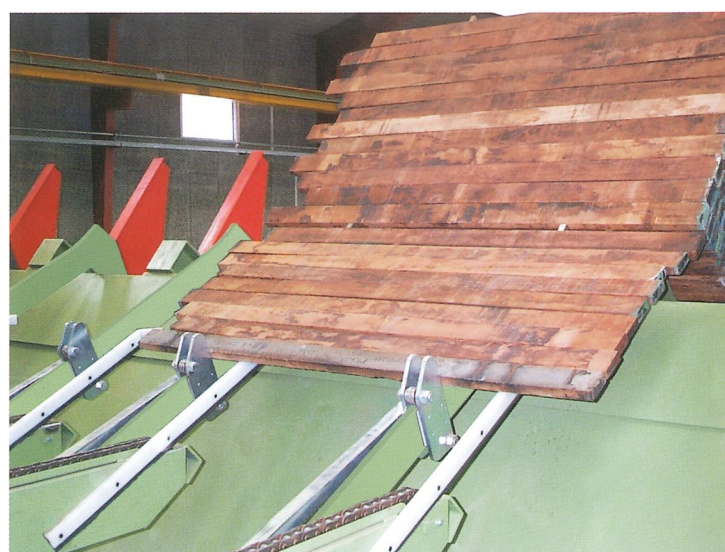
Another infeed option could be a tilt hoist infeed. For the safe and careful handling, the tilt hoist can be equipped with hold back arms, ensuring gentle and well-controlled descent onto the cross chain conveyor, reducing noise and damage to the timber.
