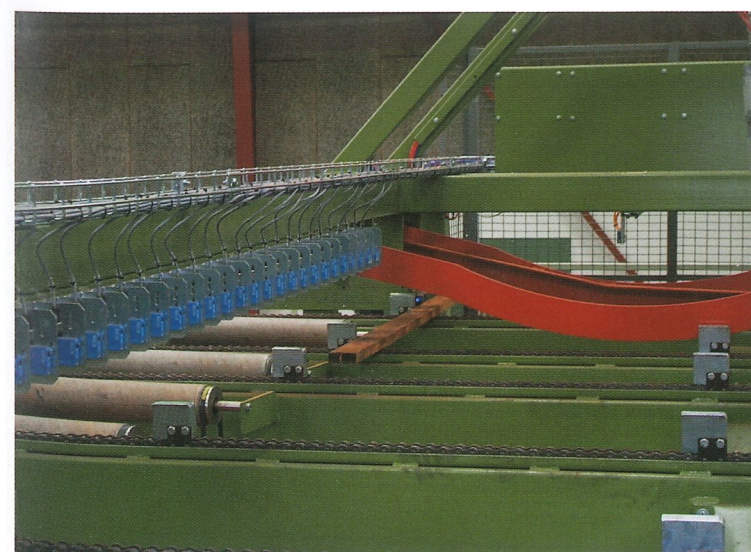
Automatic measuring of length, width and thickness of the incoming workpieces allowing you to both control your timber suppliers and to provide data for stock management ensuring a high level of traceability.
