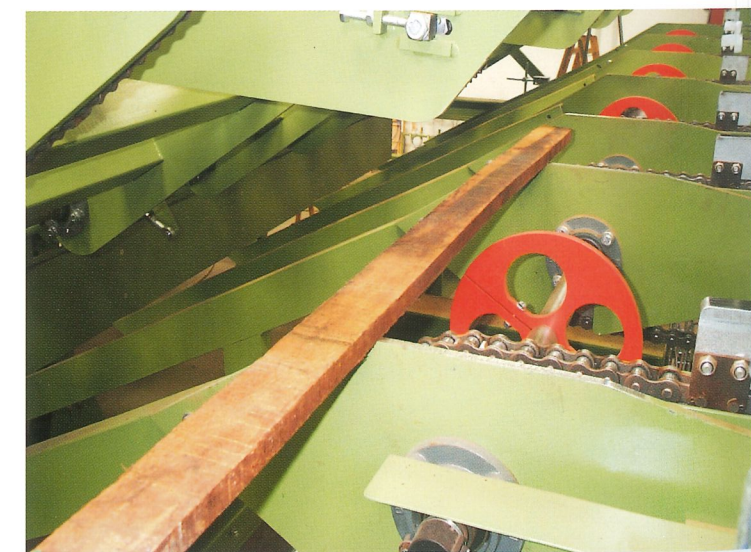
Rejecting device for rejection of workpieces or manual quality inspection. Furthermore, it can be set up for automatic sorting according to specific dimensions, if required. For rejection during quality grading, the device is operated by a joy-stick.
