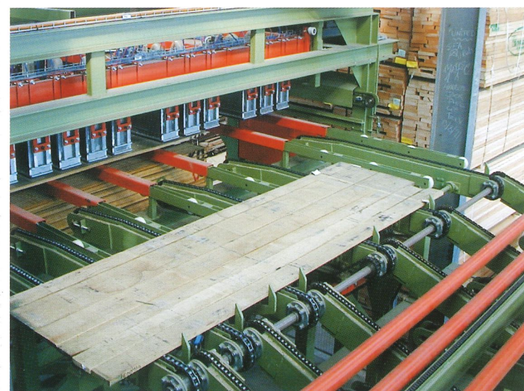
Choose between various infeed systems. Here a vacuum infeed for a very gentle timber handling without occupying too much floor space. Thanks to its flexible mounting of the vacuum heads it can adjust any distortions in the timber pack automatically.
