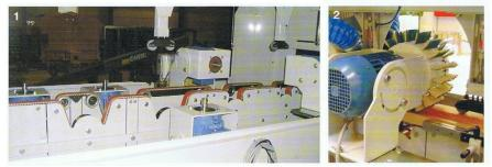
Sanding head for vertical sanding – with standard and disk sanding head.
