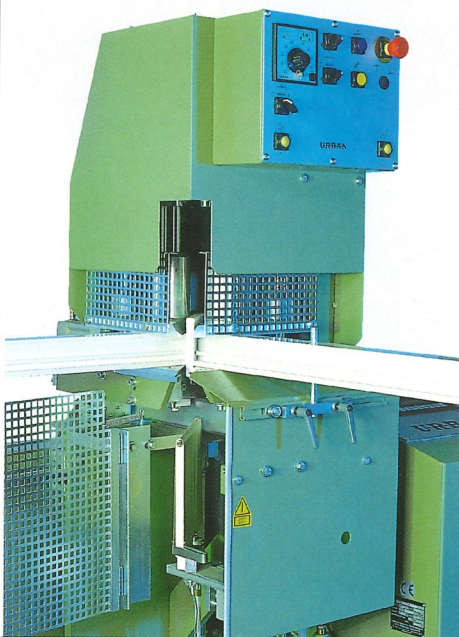
F = Winkel-schweißkopf F = Angle welding head F = Tête de soudage d'angle
