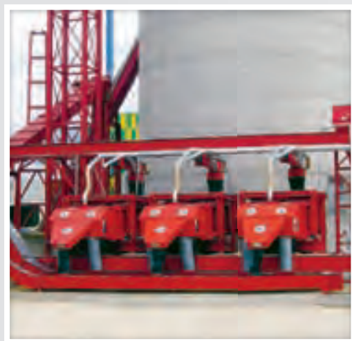
Example: Oscillation screen (VSS)
