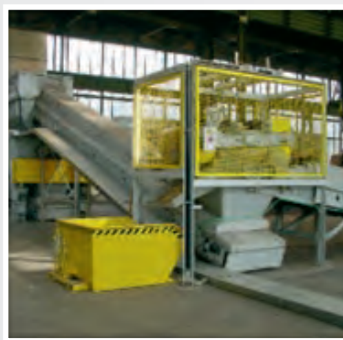
Example: Overbelt magnetic separator (VÜB)
