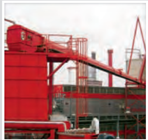
Example: Pipe belt conveyor (VecoBelt)
