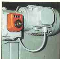
Motor and mechanic digital counter on height adjustment feeding device
