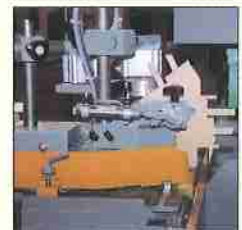
Easy to change round backing wood. Pneumatic controlled*
