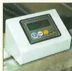
Electronic digital read-out on length-fence
