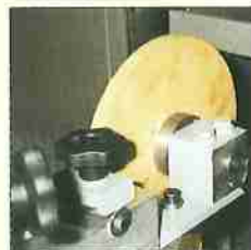
Round backing wood. 6 manual adjustable positions
