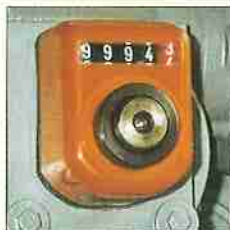
Mechanic digital counter on height adjustment feeding device
