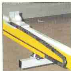
Automatic length fence with large back stop
