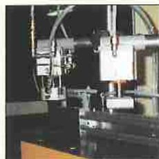
Automatic table movement with pneumatic clamps
