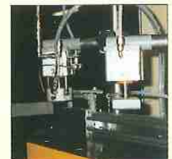
Automatic table movement with pneumatic clamps
