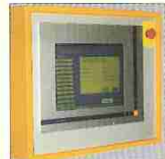
On line control. PC interface for machine control
