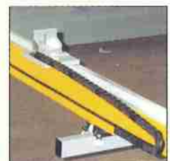
Automatic length fence with large back stop.**
