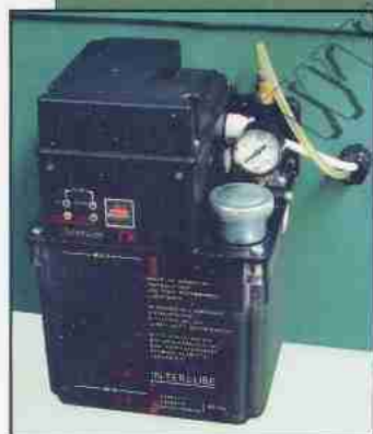
AUTO-LUBRICATION SYSTEM Comprehensive lubrication to all slideways and ballscrews.
