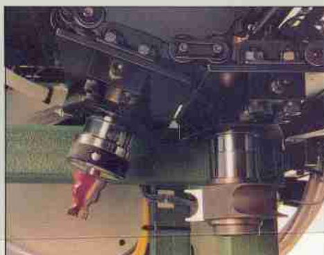
CHAIN TYPE TOOLCHANGER Additional capacity is easily catered for by insertion of extra toolholder links.
