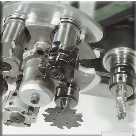
6-fold tool changer moving in X-and Y-direction
