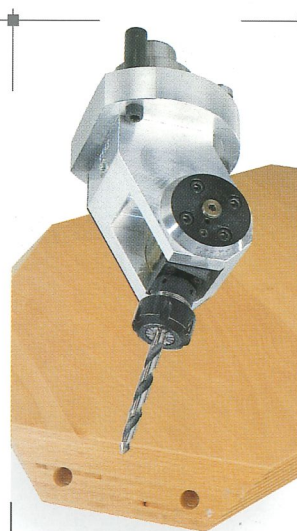
HSK 63 boring/routing inclinable For boring and sawing up to a depth of 78 mm under any angle (0°-360°). The inclination of the borer or the saw blade can be adjusted manually (0°-90°).
