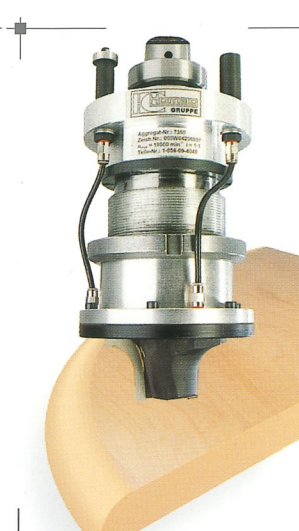
HSK 63 routing vertical with tracing ring For routing in the workpiece surface, for routing of profiles or for tongue and groove connections. The complete surface of the tracing ring can lie on the workpiece. Chips are being removed by the integrated blow nozzle. (0°-360°).
