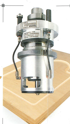
HSK 63 routing vertical with tracing ring For routing in the workpiece surface, for routing of profiles or for tongue and groove connections. The complete surface of the tracing ring can lie on the workpiece. Chips are being removed by the integrated blow nozzle.
