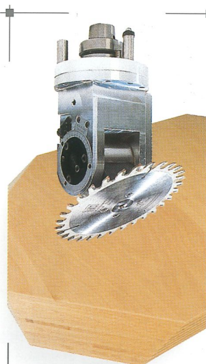
HSK 63 boring/sawing inclinable For boring and sawing up to a depth of 50 mm under any angle (0°-360°). The inclination of the borer or the saw blade can be adjusted manually (0°-90°).
