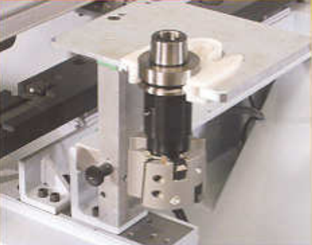
Secure and quick fitting of the tool changer
