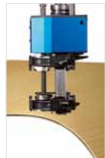
Flush trimming aggregate
