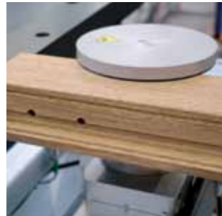
PowerClamp E.g. for processing of solid wood components from 6 sides (lowerable base plate)
