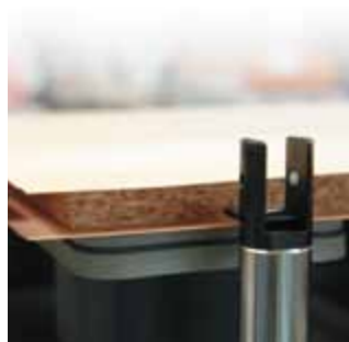
Additional tilting stops for veneer overhang Guarantee simple positioning of panels with veneer overhang
