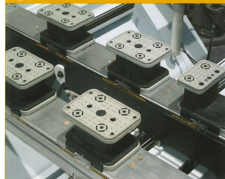
The LED-lights display the correct position of the cups to the operator. Up to 70 % faster positioning.
