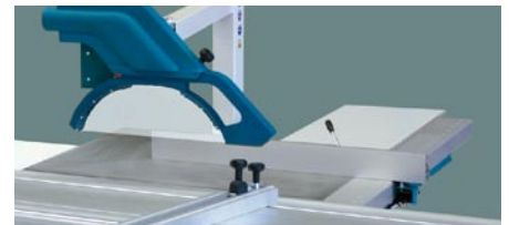
Rip fence controlled electronically
