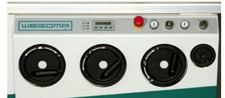
Front panel: Adjustment of height, angle and rip fence.
