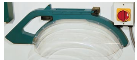
Side view of saw guard fixture
