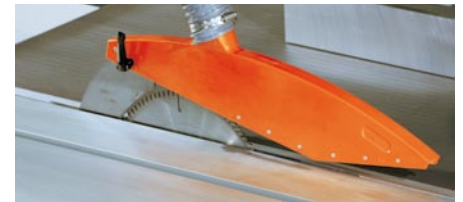
Saw guard secured to riping knife
