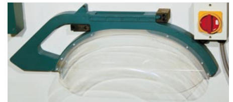
Side view of saw guard fixture.
