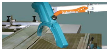
Potence d'aspiration escamotable
