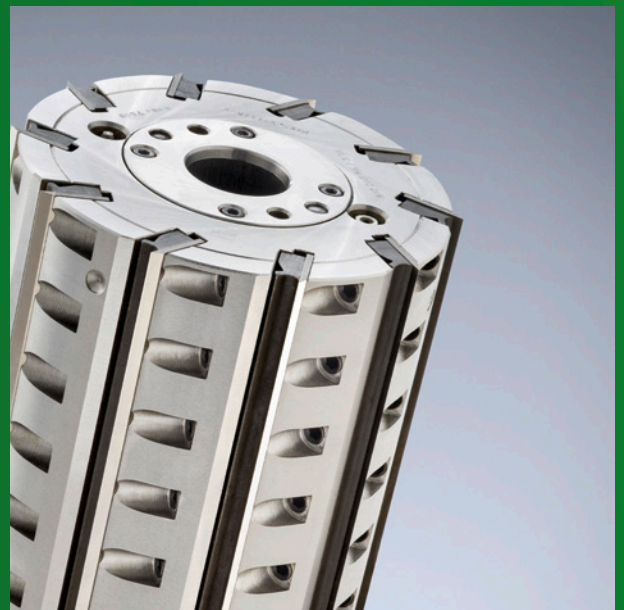
Regrinding of planer knives in the head
