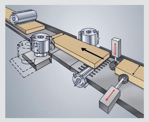
The Universal spindle is what you need for certain complicated production tasks. Usable in a 360-degree rotation, it means an additional spindle on every side and manages even the most complicated kerfing, grooving and limited profiling in a single run.
