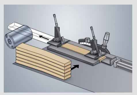
Forget complicated measuring, setting and manual feeding of every single workpiece during a straightening operation. With the automatic thickness measuring and surfacing system, just put the desired workpieces into the feed magazine and set the required thickness. Done. The precision of the system saves wood and a specialist is not needed. Pneumatic cylinders push the workpieces up to the fence and into the feed rollers.
