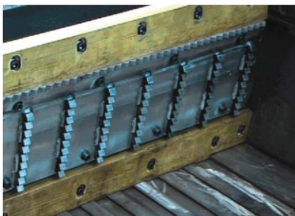
Pronged rail in the ram for holding the material
