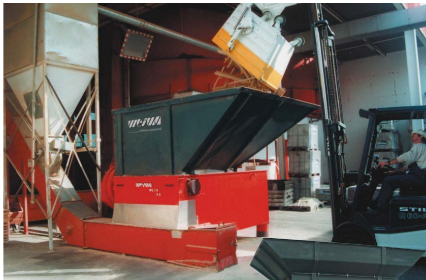
Material loading by fork-lift truck with tipper
