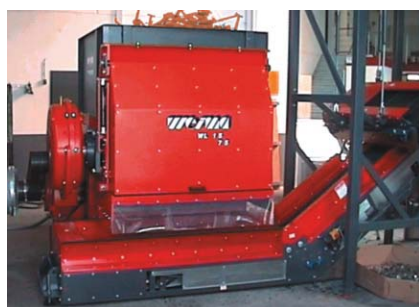
Shredder of the WL 15 series with discharge conveyor and overbelt magnet
