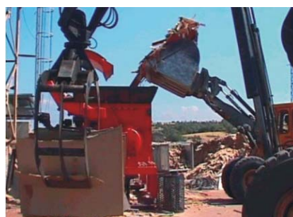
Shredder of the WL 20 series, loading by wheel-loader
