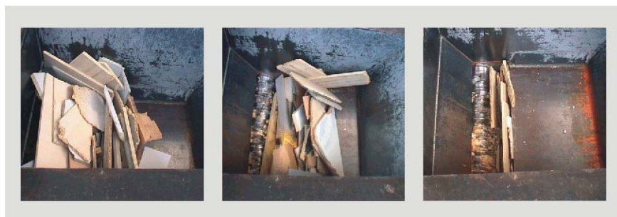
Operation of the ram, pressing the material against the rotor
