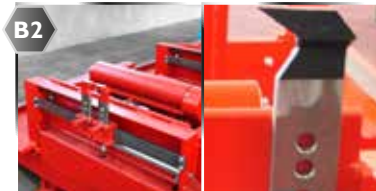
grip with two cylinders + mechanical grip lift
