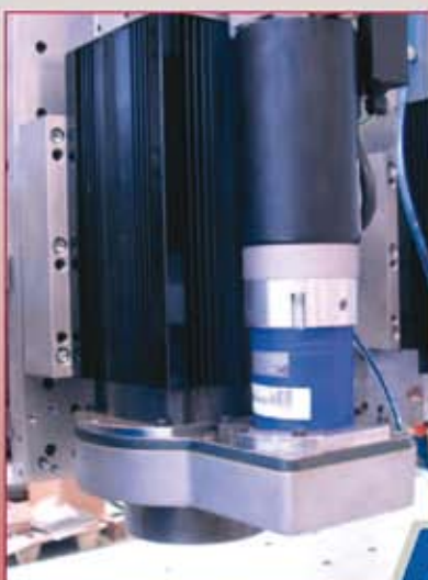
Elettromandrino con asse "C" rotante 0° - 360° Electrospindle equipped with rotating "C" axis from 0° - 360°
