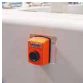
Top rollers raising through motorized spindle with analogical comparator read out.
