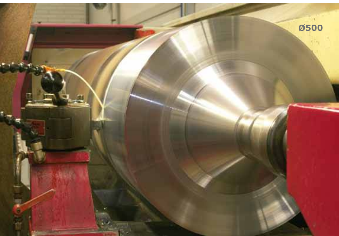
Preparation for the roller assembling Ø500.
