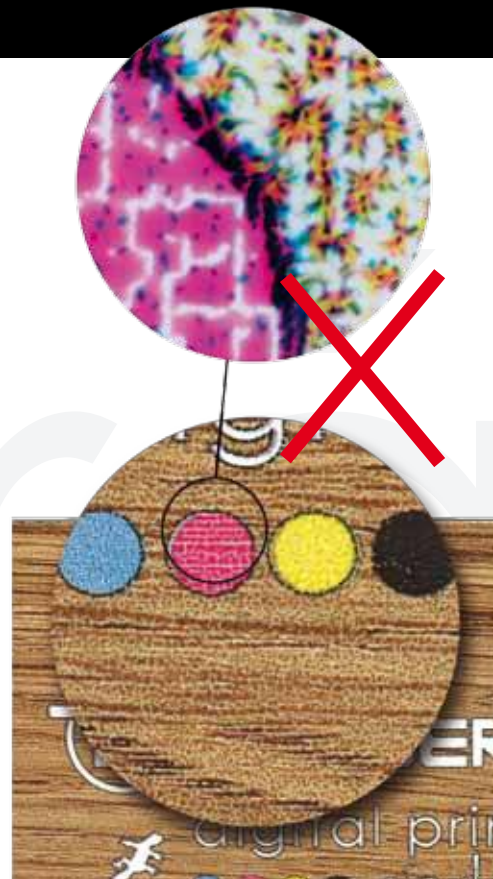
-Detail of a digital print on a substrate with unproper pretreatment.
