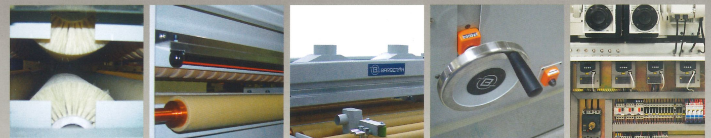
Cepillo superior y otro inferior de fibra vegetal. Machine with one upper and one lower reverse rotating brushes of vegetable bristle.
