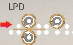
Cepillo superior y otro inferior de fibra vegetal. Machine with one upper and one lower reverse rotating brushes of vegetable bristle.
