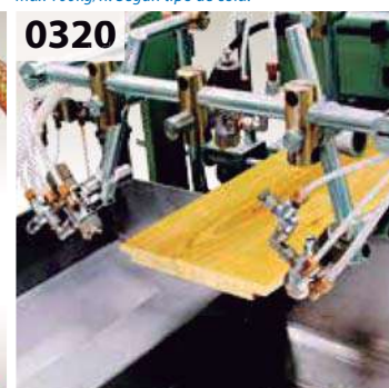
0320 3 guns + stainless pump for PVAc glue application. 3 pistolas + bomba inox. para aplicar cola PVAc.
