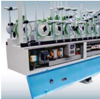
Built-in electrical cabinet. Armario dentro de bancada.
