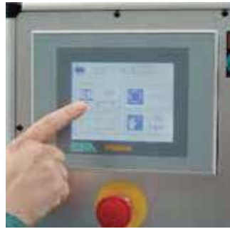
Glue grammage regulation system through PLC. Sistema regulación gramaje cola mediante PLC. (PUR)
