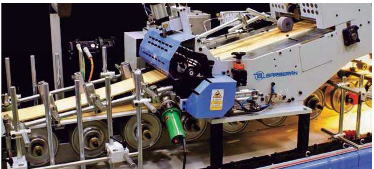
Gluing of top and bottom lath / Encolado de liston superior e inferior
