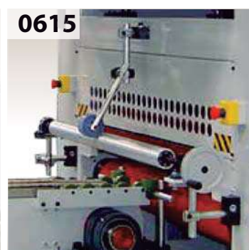
0615 Foil surplus collector to initiate the wrapping process with rolled material. Bobinador para recoger el folio inicial sin encolar.
