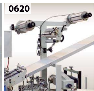
0620 Two unwinding stations with manual splicing device with air shafts. Doble desbobinadores con empalme manual (cola termofusible). Eje expansible. (PL-RP)
