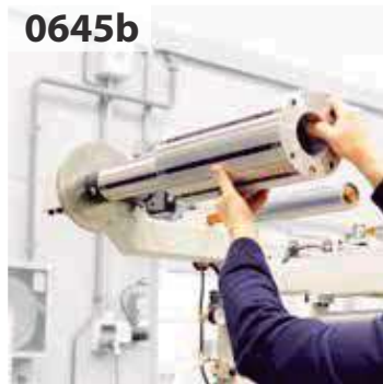
0645b This air shaft allows you to make an immediate change from an internal coil diameter of 76 mm to another of 152 mm. Permite realizar un cambio inmediato de un diámetro interno de bobina de 76 mm a otro de 152 mm.
