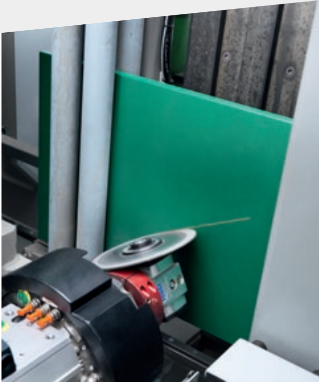
Cutting machine with integrated C-axis (optional).
