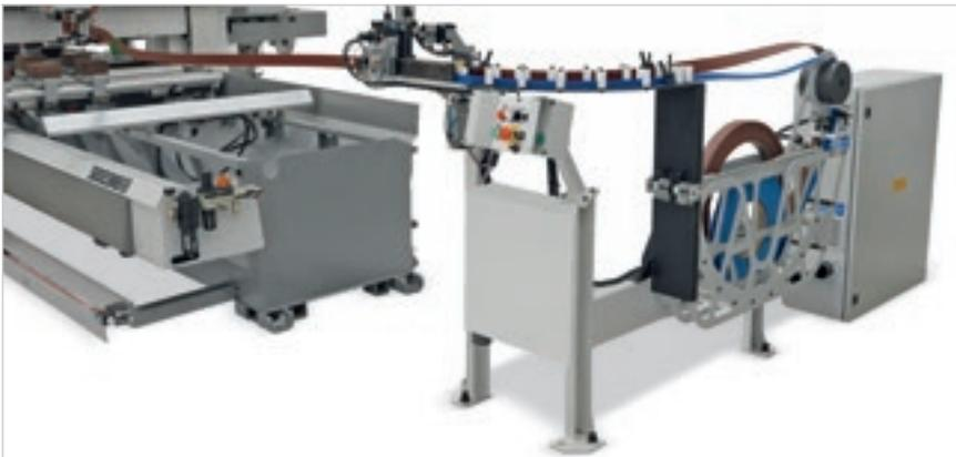
Quick change of the coils with the banding material container positioned outside the safety fences.
