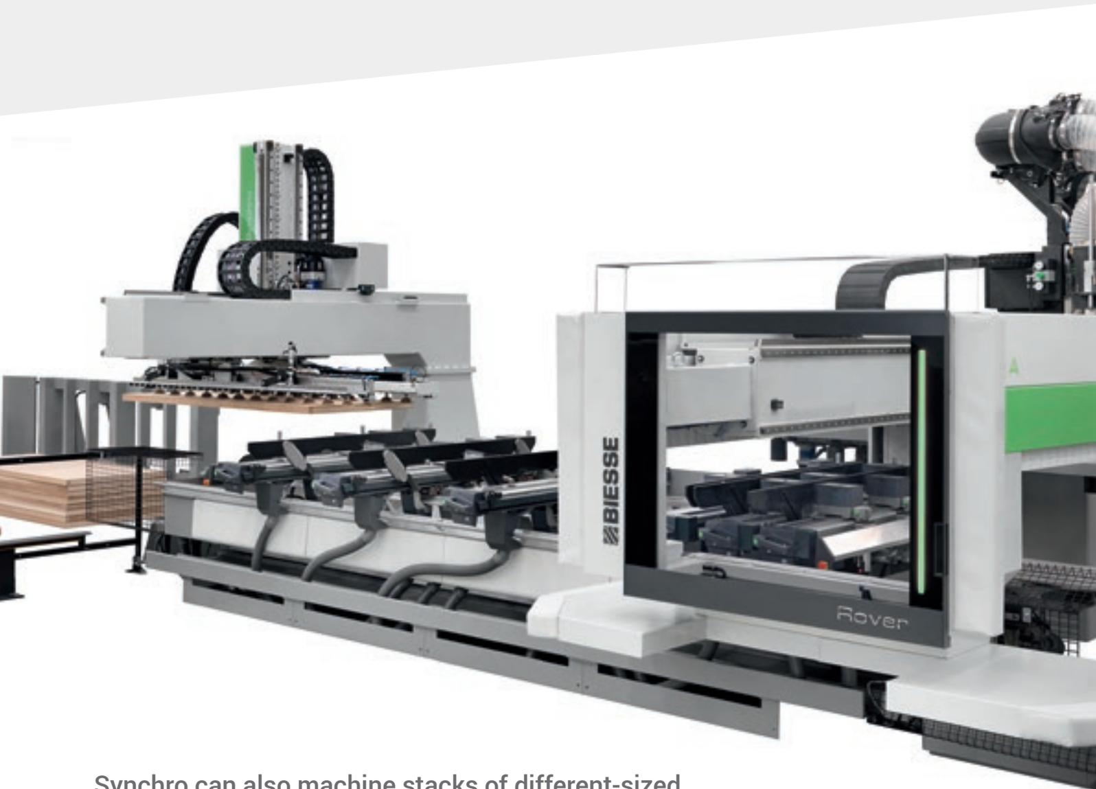
Synchro can also machine stacks of different-sized panels, thanks to stack reference device and the panel pre-alignment cycle, which is performed while the machine is running, while the Rover machining centre processes the previous panel.
