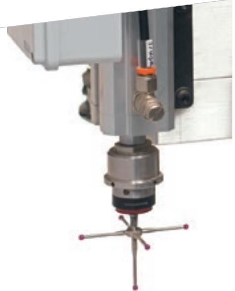
The cross-head thickness tracer enables operators to measure panel dimensions with absolute precision.
