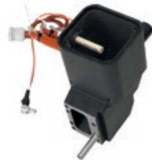
Additional glue pots fitted with quick-release electrical system for PU granule adhesives.
