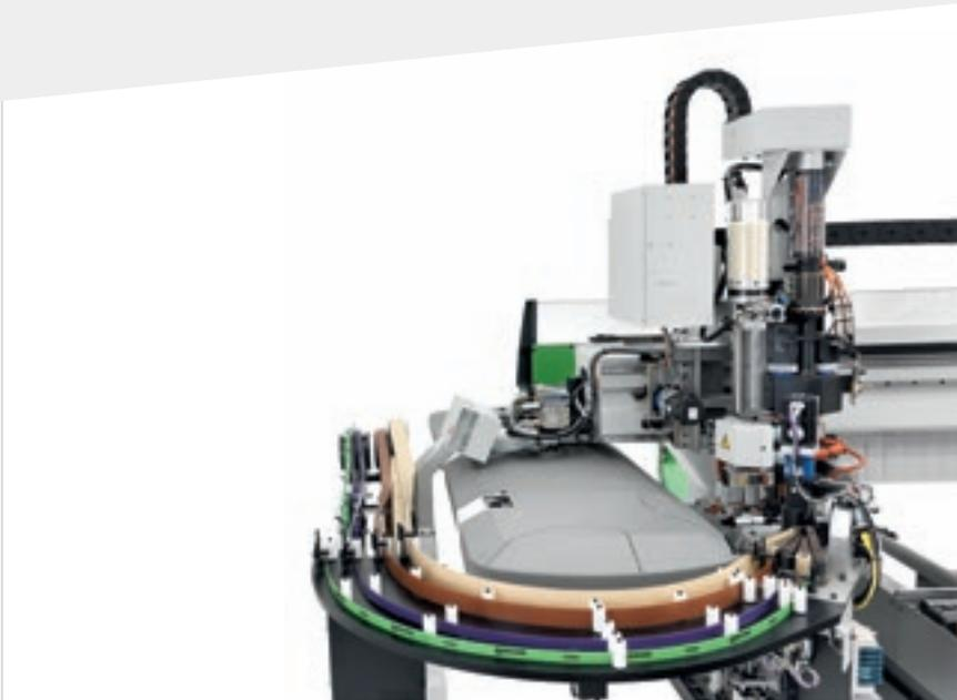
The automatic edging feeder, mounted on the X carriage, allows the user to change between thin or thicker edges during the same machining cycle.
