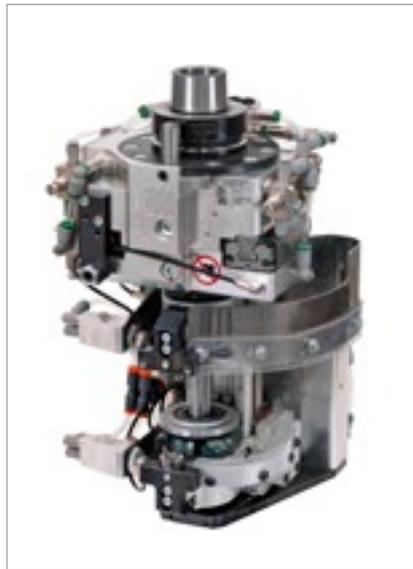
Trimming aggregate with non-stick liquid delivery.
