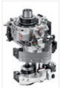
Edgebanding strip finishing aggregate with three functions: trimming, edgebanding strip and glue scraping; 30 mm minimum internal radius.
